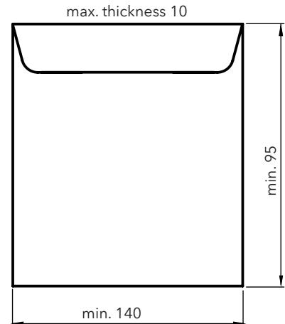
**Dimensions (mm) and weight (Matrix F42 with semi automatic feeder MFD)**
